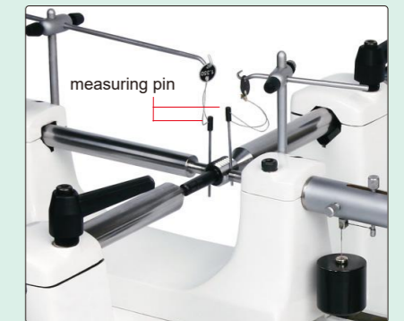
measure pitch diameter of thread
