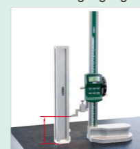
check height gauges
